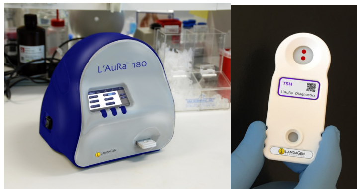
Figure 1: LamdaGen's small benchtop L'AuRa 180 digital reader (left) and cartridge (right) prototypes for rapid and quantitative POC diagnostic testing.
